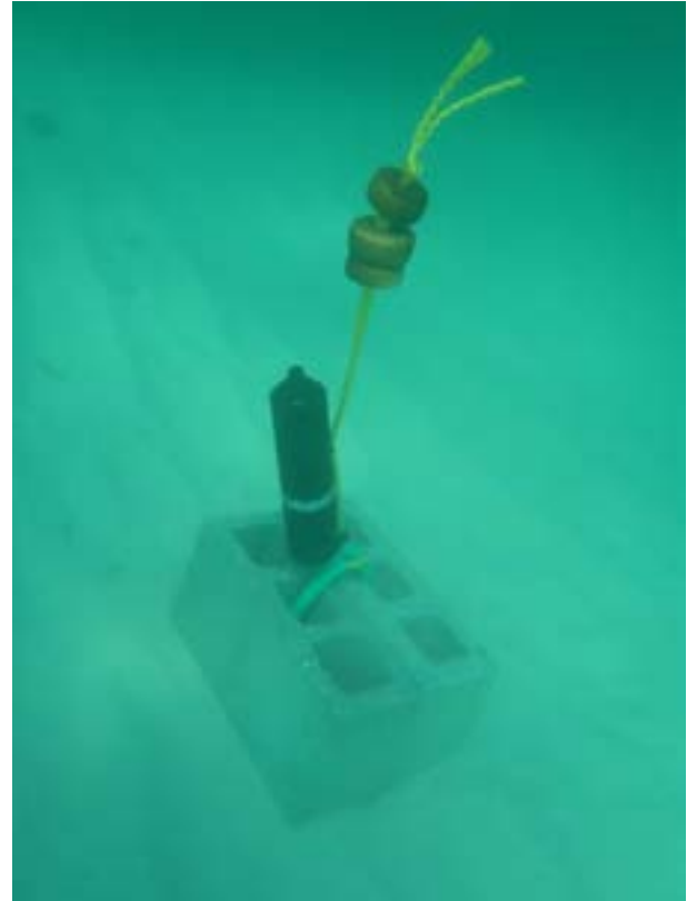
An acoustic receiver is anchored to the ocean floor and held upright with a couple floats.
