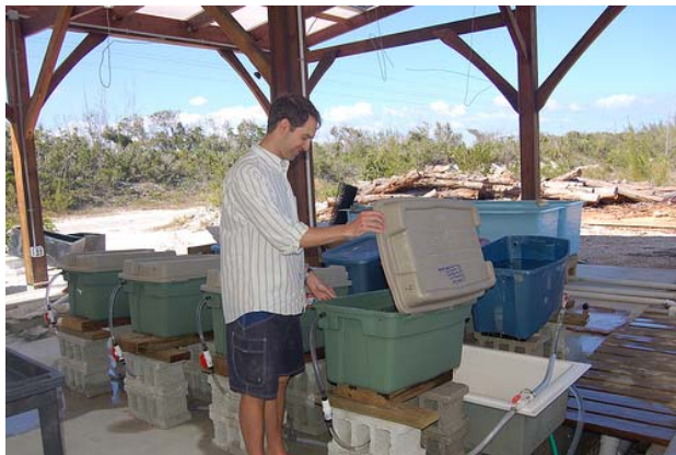
Photo 5. Fish were held in individual chambers continuously supplied with sea water for laboratory physiological studies. Here, Dr. Suski prepares to sample a fish.
